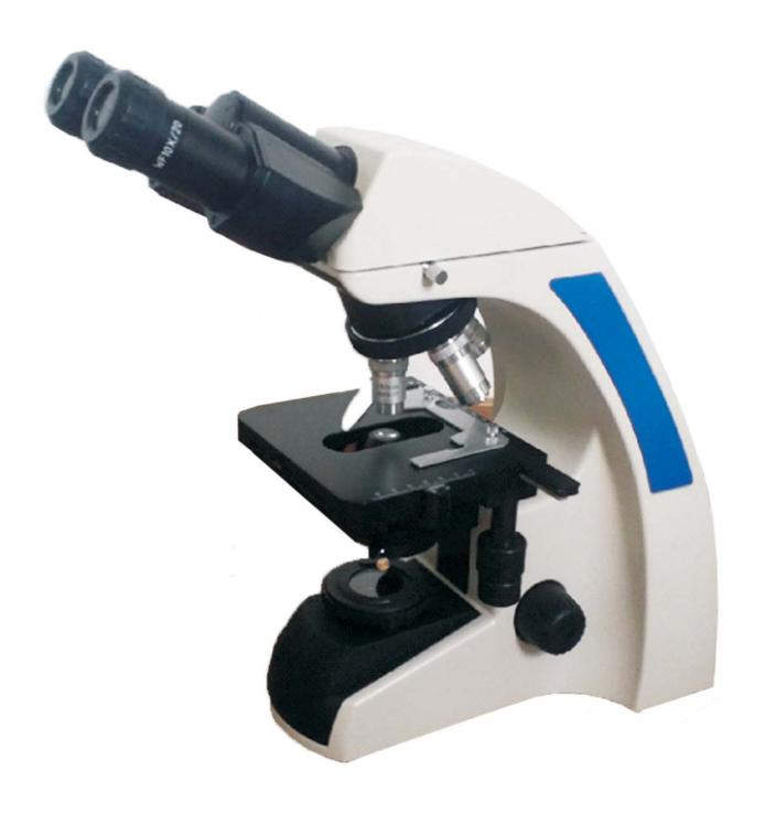
CS-U3400 is packed with powerful performance, crisp clarity and rugged construction. It's design ensures comfort and dependability for hours of daily use. The narrow front and low controls allow for arms and hands to rest flat on the table, reducing arm and shoulder strain. The rubber feet and wide rear footprint keep the microscope stable and reduce vibration for steady viewing.
